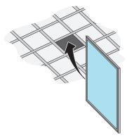
3 Make sure to angle the luminaire to get it through the ceiling opening.
