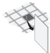
2 Lift the luminaire through the ceiling opening.
