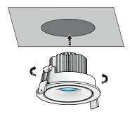
**4.)** Twist and tilt the luminaire to light up the desired area.
